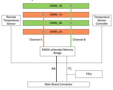
Figure 6. Memory Board Block Diagram
